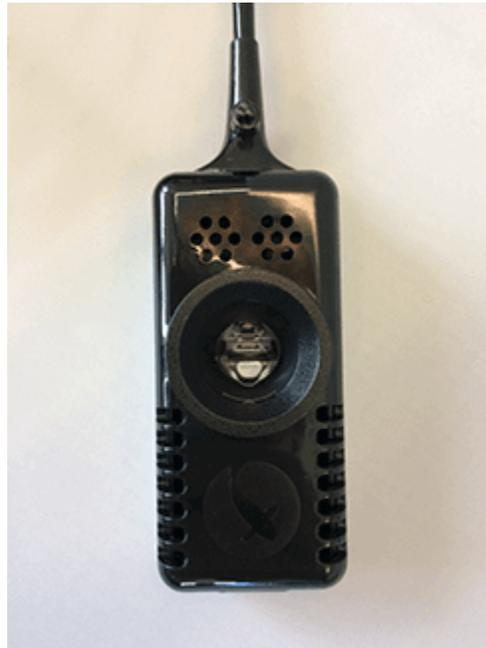
The sensor flashes a red LED through this window. Depending on if this window is covered by air or by water – and therefore if the light is travelling into a more or less dense material – the light from the LED either travels through the window or is reflected back into the sensor. The top half of the diagram below shows how light travels through the window if it is covered by water, and the bottom half shows how it is reflected back if the window is covered by air:
